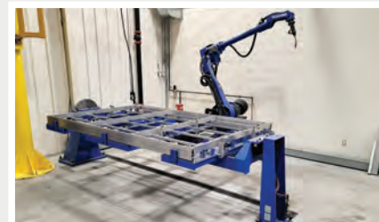
Advanced CMT Robotic Welding Technology
